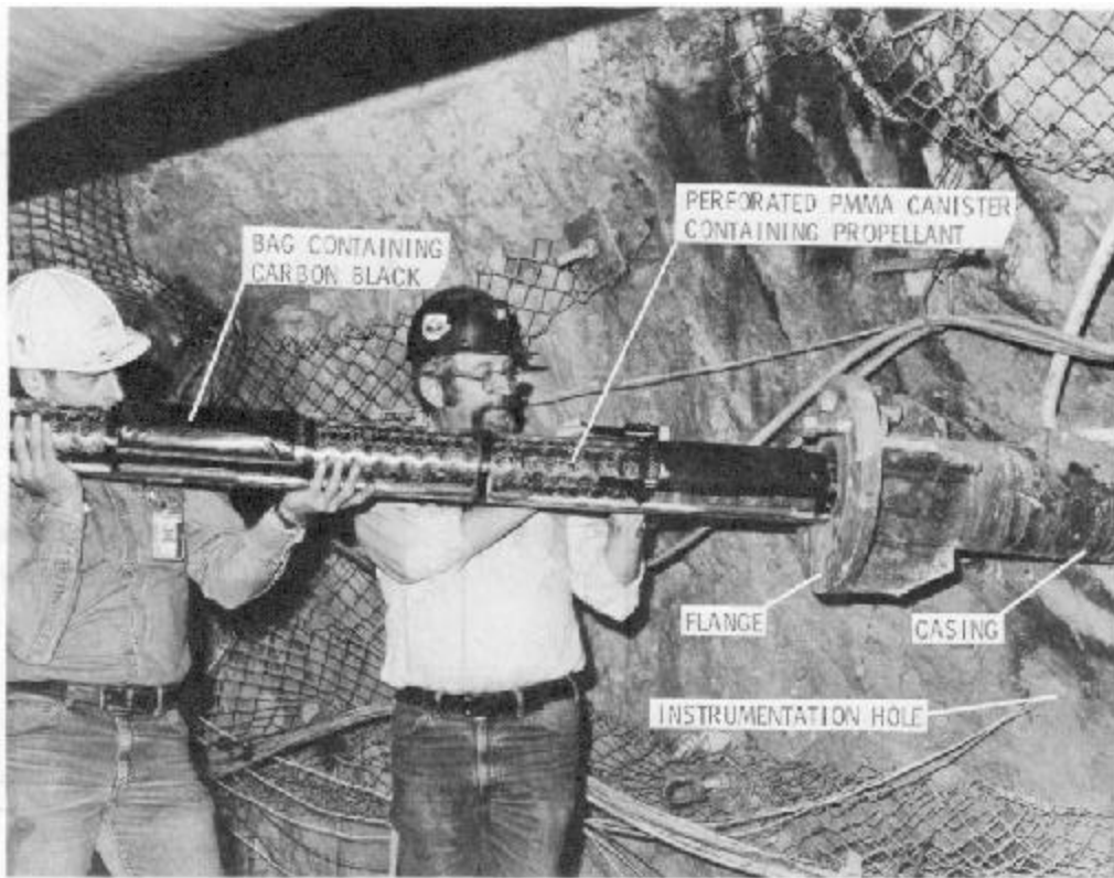
Fig. 7 - Loading of propellant device for experiment 2.
