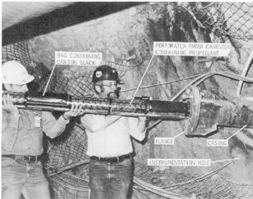
Fig. 7 - Loading of propellant device for experiment 2.
