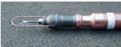
New end cap attached to GasGun tool.
